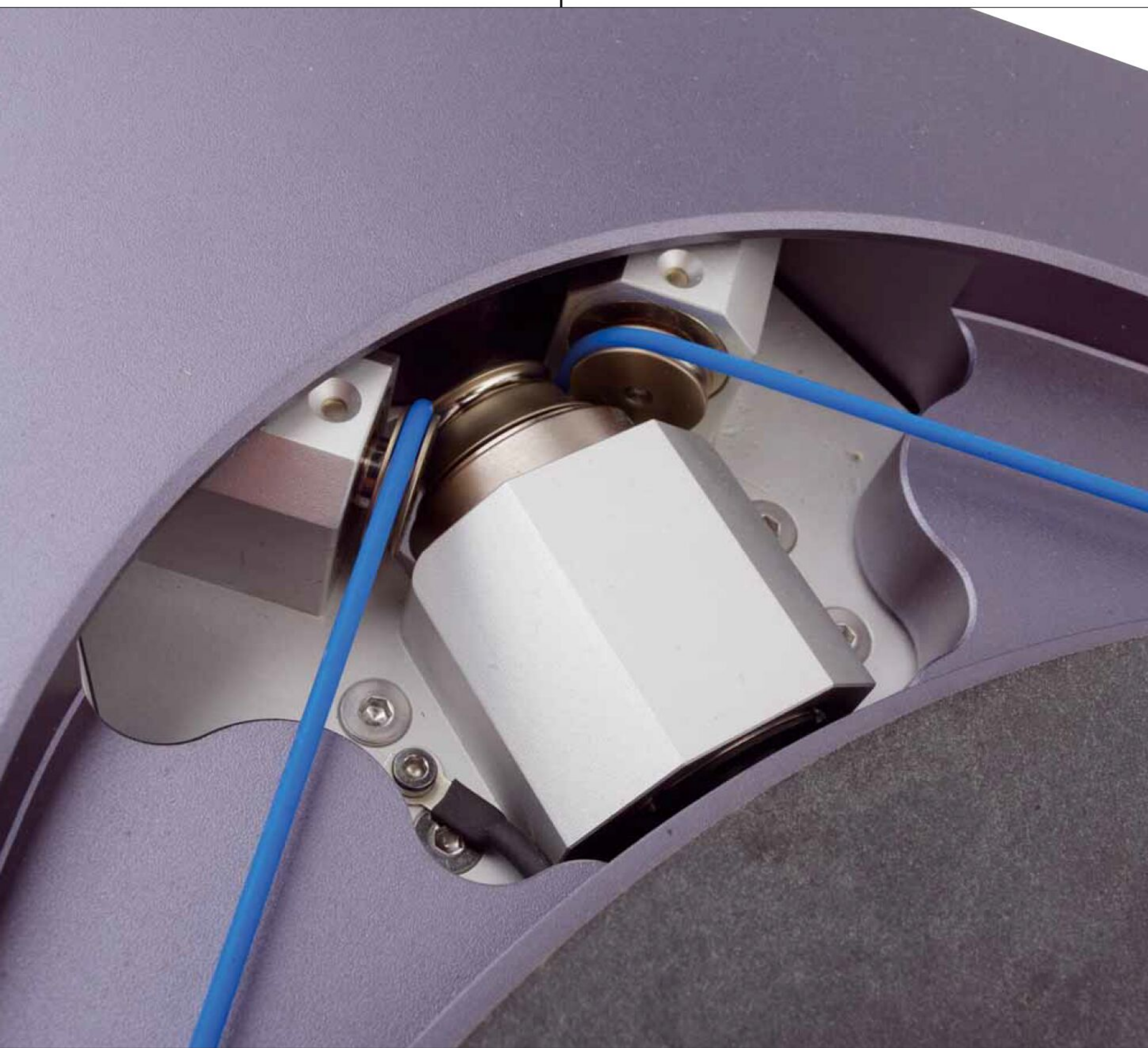
The motor axis is horizontal, which is why the belt has to be deflected twice
